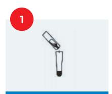
Place an extraction tube in the workstation. Open buffer tube and pour solution into the extraction tube.
