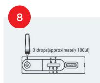
Transfer 3 drops (approx. 100UL) to the sample window of the test cassette.
