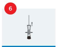
Remove the swab while squeezing the sides of the tube to extract the liquid from the swab.
