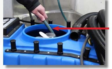
Clean out top recovery tank thoroughly, flush with clean water.
