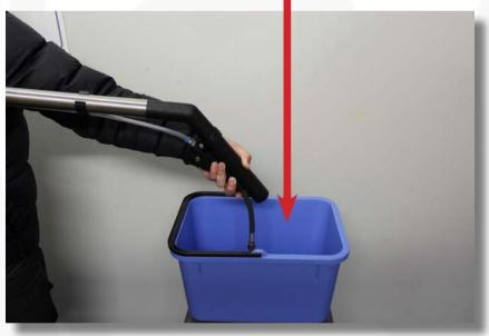
Disconnect wand from hose and turn upside down over a drain. This will empty the wand of water to keep it in good condition when not in use. 2.
