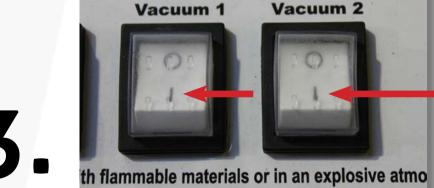
Run vacuum for 10 minutes with the top dome removed. This will dry out any moisture that is sitting near the motor.
